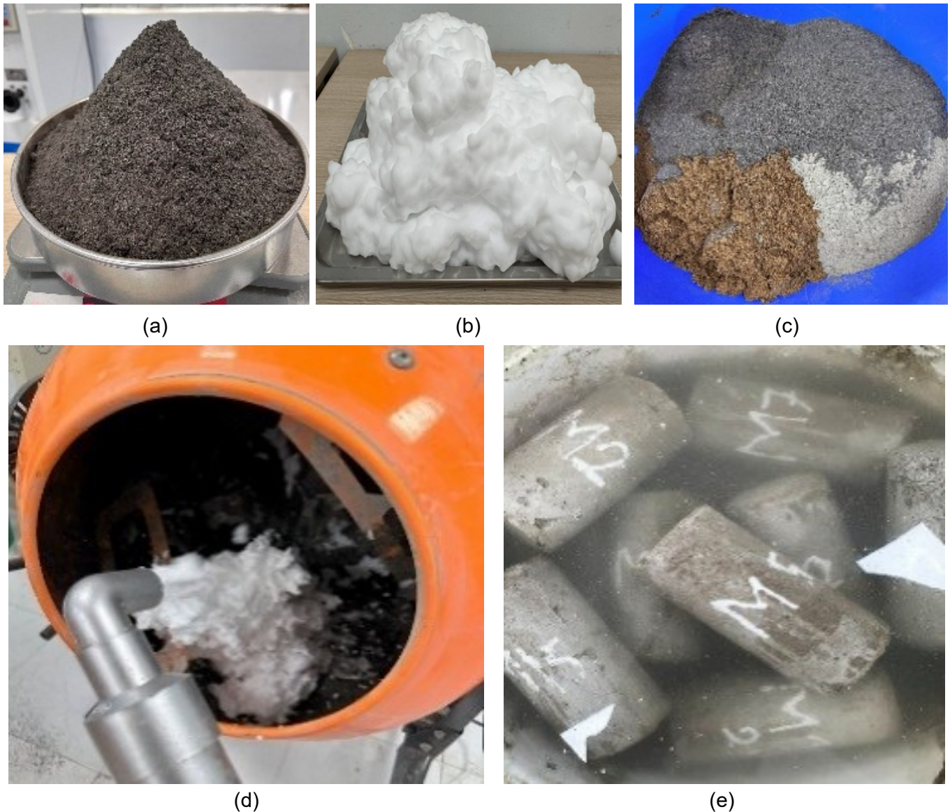
Fig. 1. (a) IBA; (b) generated foam; (c) mixing components; (d) casting foam into slurry; and (e) curing of specimens
