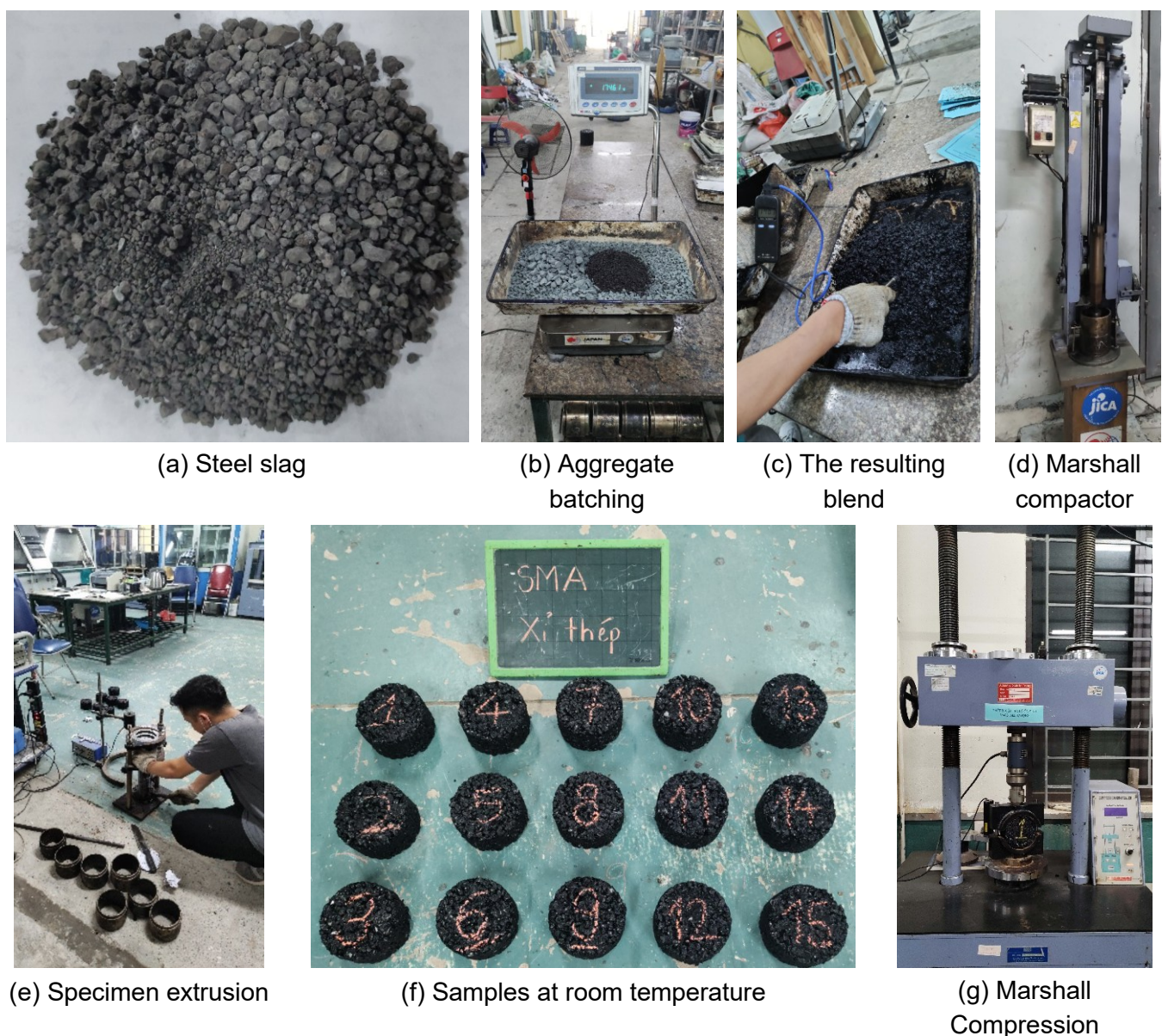
Fig. 1. Marshall test procedure for SMA mixtures
