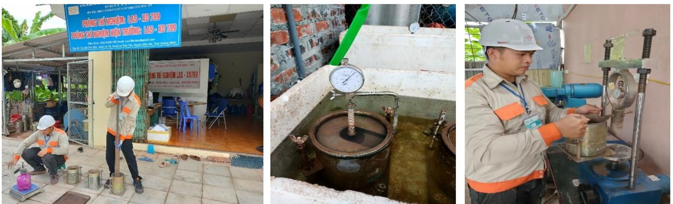
**Fig 3.** Testing work of California Bearing Ratio (CBR) of Laboratory-Compacted Soils
