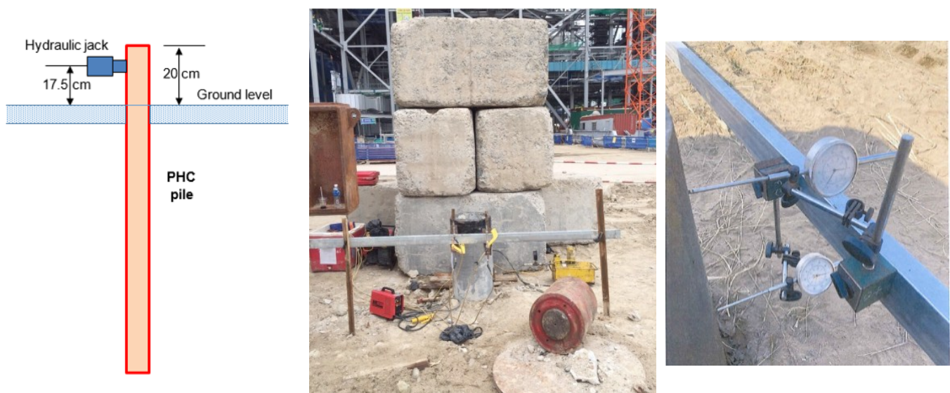
Fig. 2. Installation diagram of lateral test pile
