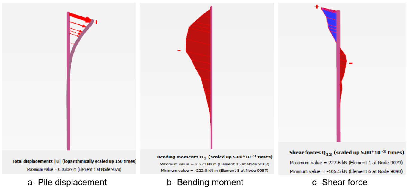
Fig. 5. Analysis results of pile L500-01 using the Plaxis 3D model
