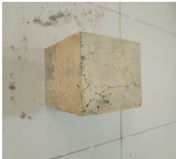
Fig. 8. Destructive form of specimens in the Group G3
