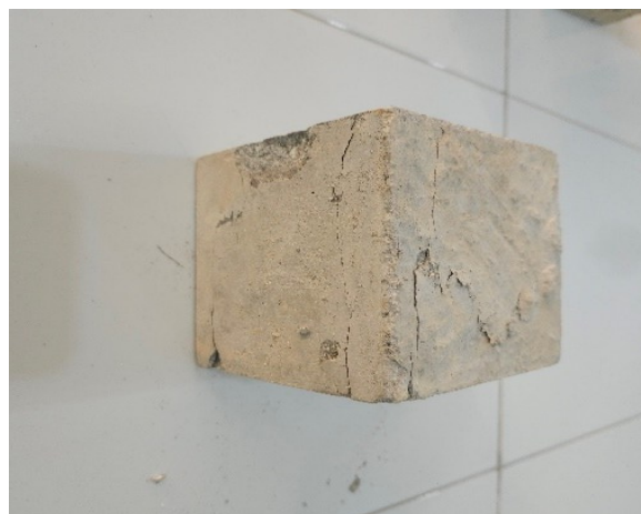
Fig. 7. Destructive form of specimens in the Group G2
