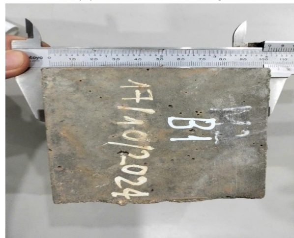
(f) Specimen dimension check
