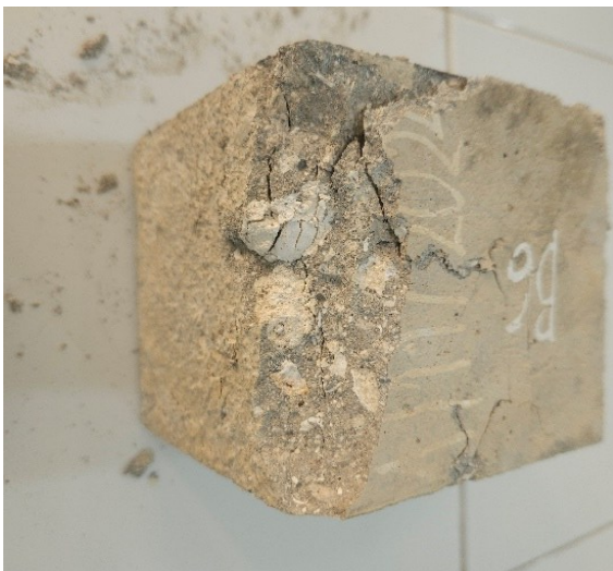
Fig. 12. Destructive form of specimens in the Group G7
