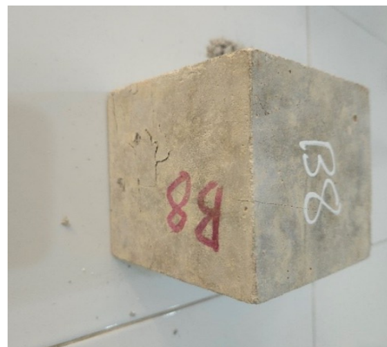
Fig. 9. Destructive form of specimens in the Group G4
