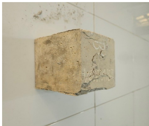
Fig. 10. Destructive form of specimens in the Group G5
