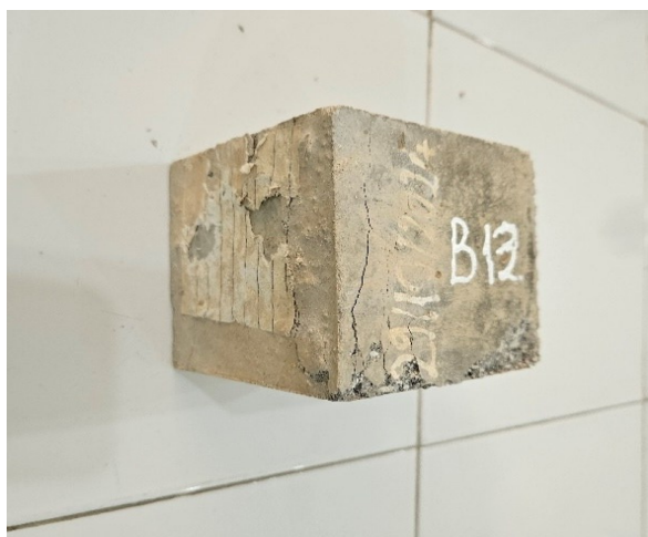
Fig. 6. Destructive form of specimens in the Group G1
