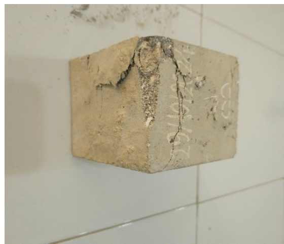
Fig. 10. Destructive form of specimens in the Group G5
