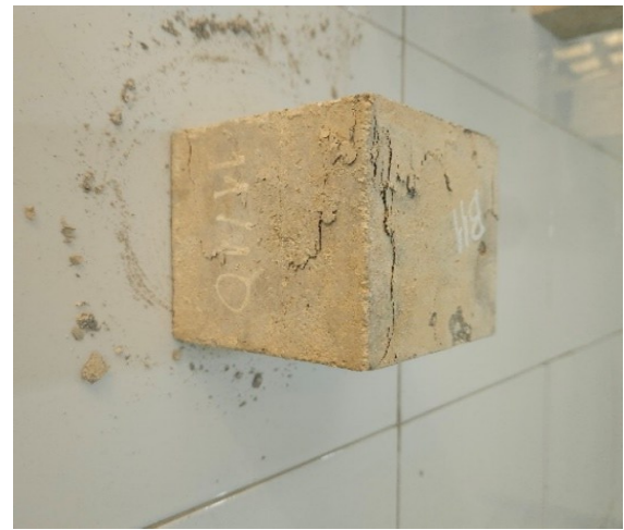
Fig. 11. Destructive form of specimens in the Group G6
