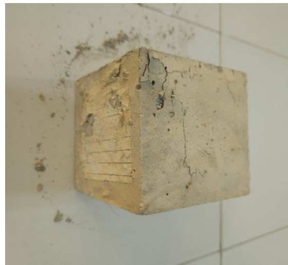
Fig. 8. Destructive form of specimens in the Group G3
