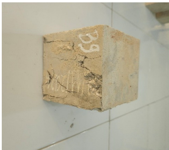
Fig. 9. Destructive form of specimens in the Group G4
