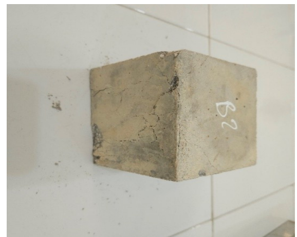
Fig. 7. Destructive form of specimens in the Group G2
