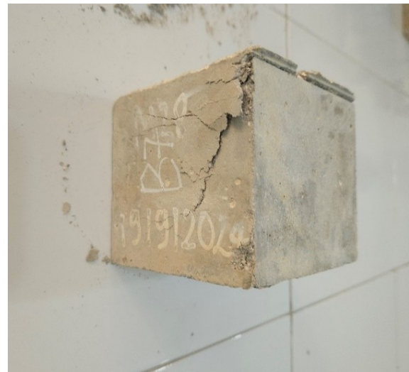
Fig. 12. Destructive form of specimens in the Group G7
