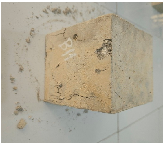
Fig. 11. Destructive form of specimens in the Group G6
