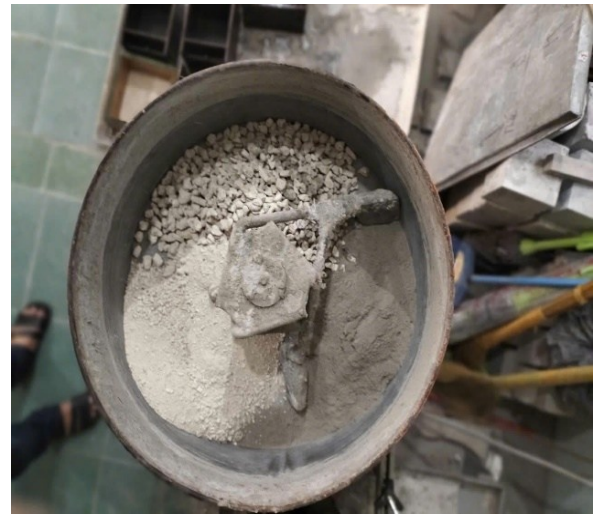
(b) Dry mixing process
