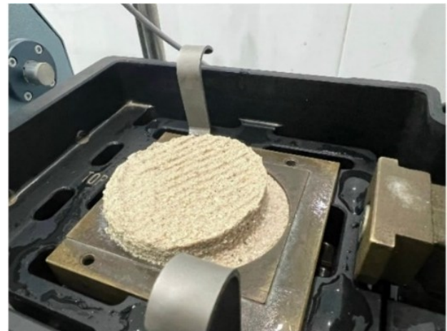
Fig. 8. Coral sand sample after completion of a shear test
