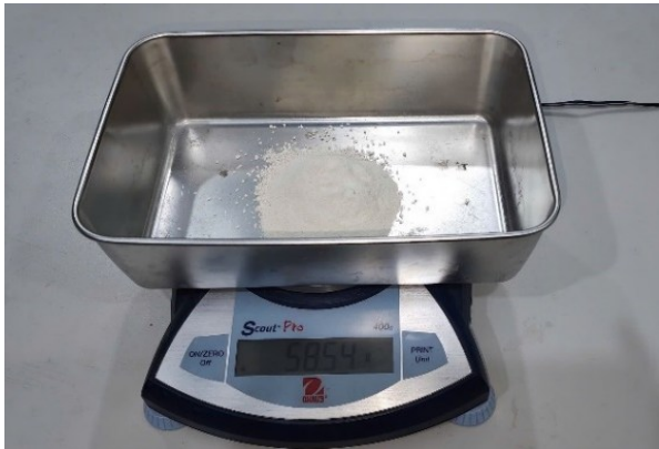
Fig. 5. Weighing the coral sand for sample preparation
