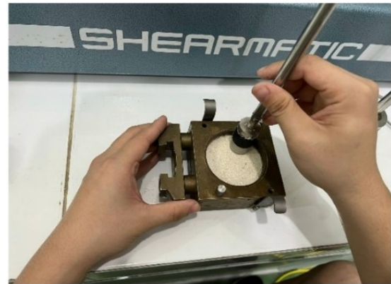
Fig. 6. Compacting the coral sand within the shear box
